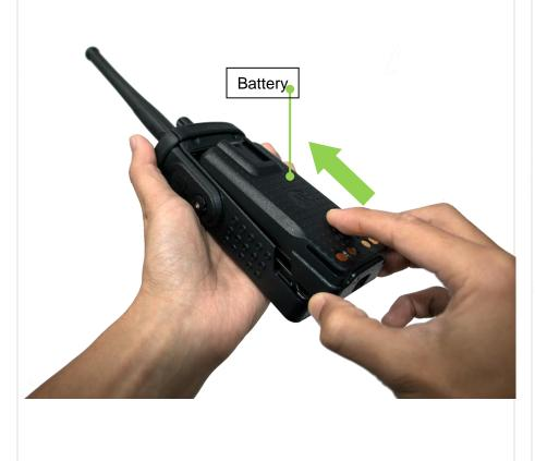
To remove the battery, turn the radio off. Lift up the latch then slide the battery down to remove the battery from the radio.
